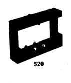
They were provided with milled slots for attaching to the table with the long side down. We have modified these things so that they can be attached to the table on the short side, or attached to magnetic bases, or supported between a pair of "goalposts".
