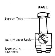
EMCO: These are from a company which distributes products from the Far East. We have samples of two catalog numbers. The smaller ones seem to be losing their handles, so if you see any floating around the lab, put them with the bases or in a MISCELLANEOUS METAL PARTS box. The magnets weren't so strong to begin with, and some of them it's hard to tell if the magnetic field is on or off, so reserve the use of these bases for lightweight
