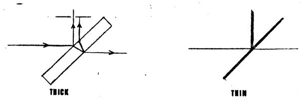
is fine for object beams, but these two reflected beams cannot be used as a reference beam because the hologram would require those same two beams for playback.
