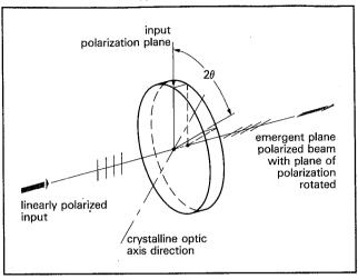
HALF-WAVE PLATE EFFECT ON LINEARLY POLAR-IZED LASER BEAM. The plane of polarization of the beam can be rotated at will without rotating the laser. The plane of polarization is essentially reflected in a plane containing the crystalline optic axis, and the output plane rotates at twice the angle rate of the retarder.
