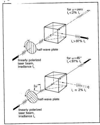
VARIABLE RATIO BEAMSPLITTER: The half-wave plate rotates with angular velocity  $\omega$  while the permitted plane of output polarization (here suggested by lines on the highly transparent retarder) rotates at angular velocity  $2\omega$ . The polarized beams which finally emerge from the cube have the irradiances  $I_s$   $I_p$  indicated. Intermediate irradiances are seen at intermediate times.
