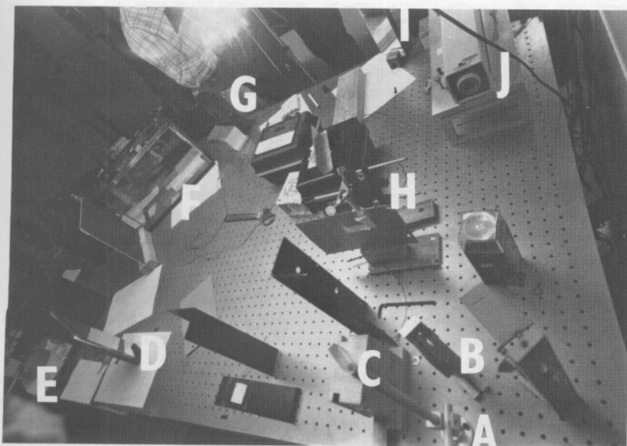
Setup for single-pulse Light in Flight recording at Northwestern University. The beam from the Nd:YAG laser comes out of the pipe at A, is turned 90° by a steering mirror at B, and is split in two by a glass block at C, with the transmitted light being expanded by lenses at D and steered by mirror E through the aquarium tank at F, where the backlit objects are placed. The object light travels on to the holographic plate holder at G. The weak reflection from the beamsplitter is expanded by lenses at H and guided to the plate holder by mirror I. The beam from a 5mW HeNe laser is used for alignment and joins the YAG beam by sneaking in from behind the dielectric mirror at B.
