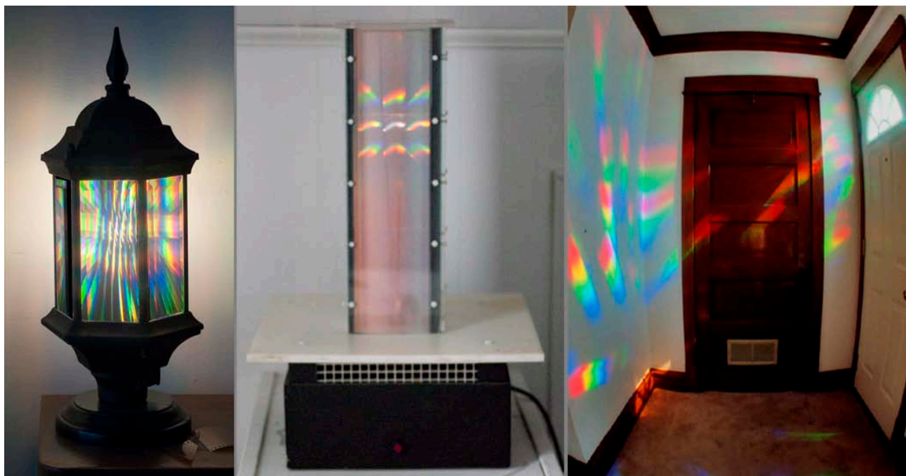
Figure 4: Pure light. Left, "Coach Lamp A", diffraction gratings surround an incandescent bulb creating a cookie jar of spectra; "The O-tron", rainbows tag along for the ride on the spark of a Jacob's Ladder's surrounded by diffraction gratings; "Rainbow Projecting Transom". diffraction gratings in my front door on a sunny morning.
