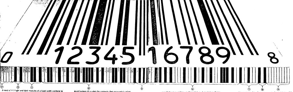
A total of 113 light and dark modules of a fixed width combine to form the bars, spaces, and margins that make up a typical UPC bar code. The modules represent individual zeros (light) and ones (dark) that express, in a computer's binary language, the bar code's twelve decimal digits, which also appear in their familiar atabic form. A border area called the quiet zone takes up the symbol's first nine modules (1), after which comes a three-module
