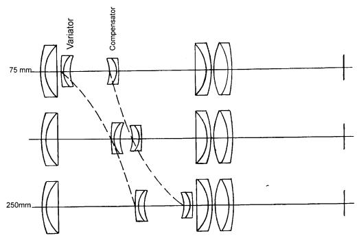
One way to make a zoom lens. As the Variator, a negative lens, moves away from the fixed positive front element, the focal length of the combination changes. The Compensator moves in response to this focal length change to maintain the focal plane's position.
