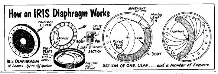
Most cameras manufacturers try to get away with as few iris blades as possible. You may notice 5 or 6 bladed irises in the typical 35mm camera lens, and even as few as three in some cheaper items.
