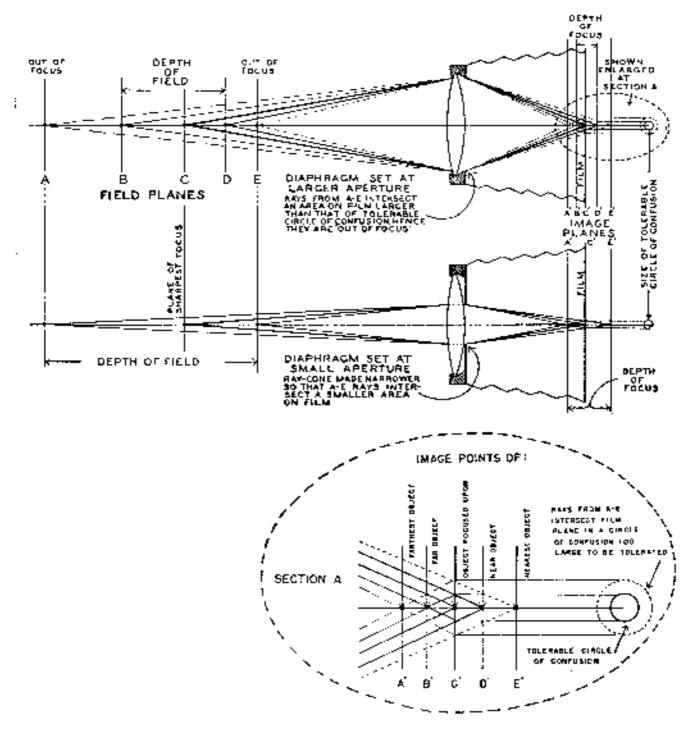
If the focused object distance is u, the focal length of the lens is F, the diameter of the lens aperture is A, and the "circle of confusion" on the film (which is a circle so small as to be indistinguishable from a point) is c', then the near and far depths of field are given by:
