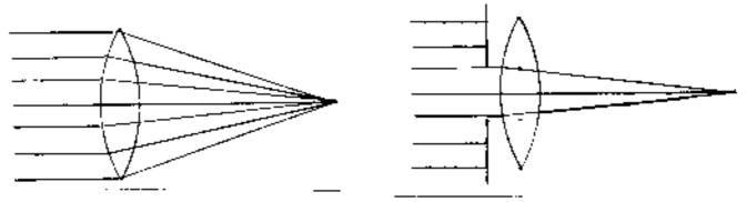
Lenses of different diameters and focal lengths can deliver the same amount of light if they all form the same tip angle of the cone of convergent light, as shown in Figure Four.
