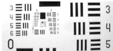
10X Lens: Resolution dies by Group 3, Element 2.
