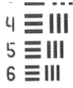
60X Lens: Resolution dies by Group 5, Element 4.
