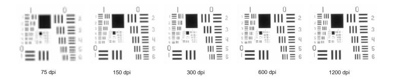
Figure X: Here is the USAF target as scanned in by a CanoScan D 660U at a variety of resolutions. They all have been resized to 1200 dpi, and are printed at 600 dpi. None of the targets are life-sized, The 1200 dpi is twice life size, 600 4X, 300 8X, 150 16X, and the 75 is 32X. You can watch how the resolution improves
