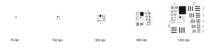
Figure X: Here is the USAF target as scanned in by a CanoScan D 660U at a variety of resolutions. They are printed at 600 dpi. The only target that is life sized is the 600 dpi. The 1200 is twice life size, , the 300 is half, 150 a quarter and 75 an 8th.
