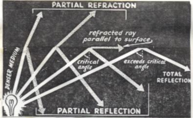
Since this is impossible, the light is perfectly reflected at the border at this first angle, the Critical Angle, and all angles greater than it will also cause the light to become trapped. This phenomenon makes fiber optics, retroreflectors, corner prisms, etc., work.
