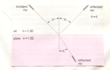
The Critical Angle is the first angle which traps light inside a slow moving medium thanks to Total Internal Reflection. light tries to escape a medium with a refractive index greater than the surrounding medium, the exiting light is bent away from the normal. When a certain incident angle value is plugged into Snell's Law, the refracted angle turns out to be 90 degrees.
