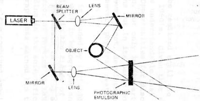
In that region of space where the two coherent beams interfere, a photographic emulsion is placed. All this is shown above in the sketch. The emulsion then records the interference pattern of the two beams. The emulsion—a black and white type of very fine grain—is developed in the ordinary way (developer, stop bath, etc.) and the first step is complete.
