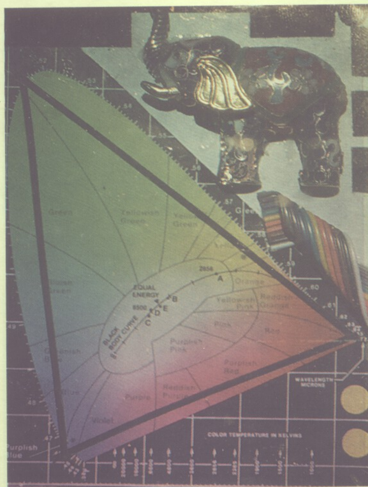
Figure 6. A 10 \times 12 -cm color hologram of the test object. The hologram was recorded with 488-, 532-, and 633-nm laser wavelengths. Note the rainbow ribbon cable, the pure yellow dots, the full range of colors, and a balanced white in the center of the CIE color test target.
