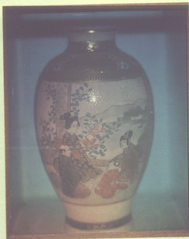
Figure 8. A 10 × 12-cm color hologram of a polychrome vase. The hologram was recorded with 477-, 532-, and 633-nm (blue, green, and red) laser wavelengths.
