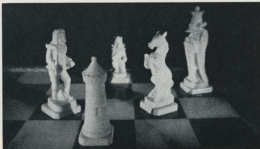
RECONSTRUCTED IMAGE was made by directing a laser beam through the hologram. The reconstructed waves were then passed through a lens and brought to a focus, thereby forming an image of original scene, even though chessmen had long since been removed.
