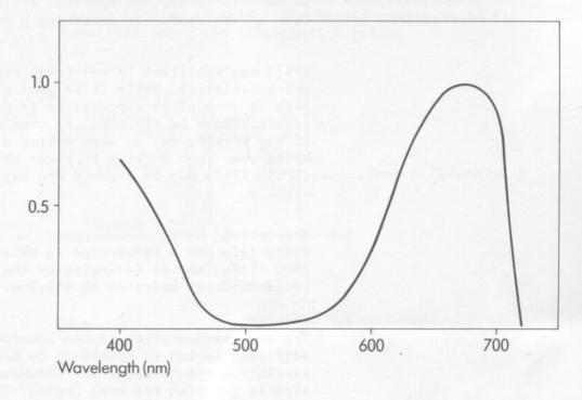
The above curve shows the relative spectral sensitivity of SP673 to white light flash exposure  $(10^{-4}s)$ . This curve shows that SP673 has a maximum sensitivity at 694nm.
