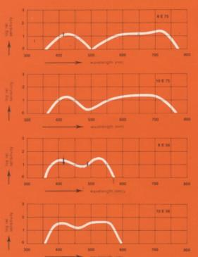
Spectral sensitivity for an equi-energetic spectrum
