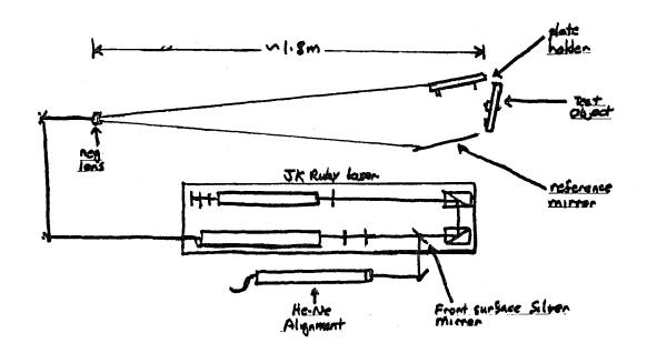
Fig 3 Denisyak Sotup for Pulsed Ruby Tosts
